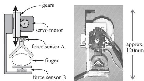
Figure 3: Apparatus's Fingertip Pressing Subsystem
