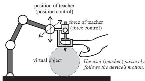
Figure 1: Proposed Mechanism — Haptic Device with Fingertip Presser
