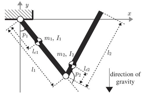
Fig. 2. 2-DOF manipulator for the simulation. ( $l_1 = 0.26$  m,  $l_{c1} = 0.0983$  m,  $l_2 = 0.26$  m,  $l_{c2} = 0.0229$  m,  $m_1 = 6.5225$  kg,  $m_2 = 2.0458$  kg,  $I_1 = 0.1213$  kg·m<sup>2</sup>,  $I_2 = 0.0116$  kg·m<sup>2</sup>. All of these parameters are the same as those in p. 115 of Kelly *et al.*<sup>10</sup>)
