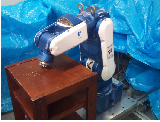
Fig. 12. Experiment III: slave robot in contact with the external environment (a wooden shelf).
