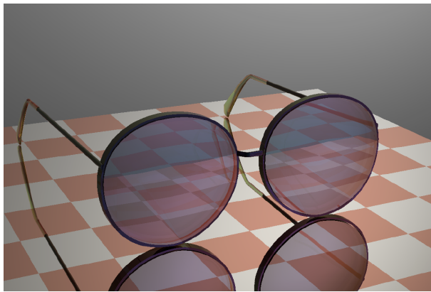
(b) glass coated with 300nm dielectric and 5nm aluminum films
