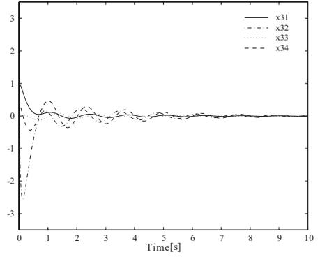
Fig. 6. Response of the closed-loop system 3 with the LQR.
