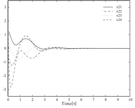
Fig. 5. Response of the closed-loop system 2 with the LQR.
