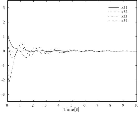
Fig. 3. Response of the closed-loop system 3 with the proposed control method.
