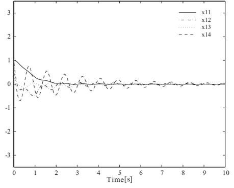
Fig. 4. Response of the closed-loop system 1 with the LQR.
