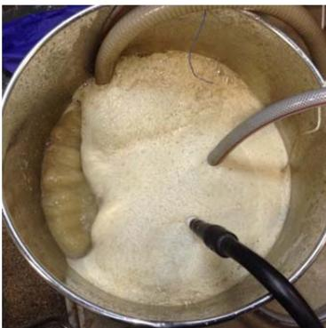
Excess sludge treatment using ozone-nanobubble
