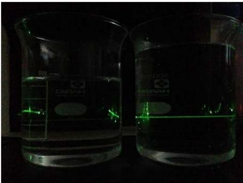
Observation of UFB using Tyndall scattering, Left: control(tap water), right: UFB water (made from tap water),
