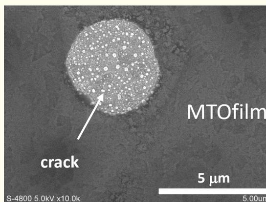
Fig. 1 Surface morphology of magnesium-tin oxide (MTO) film
