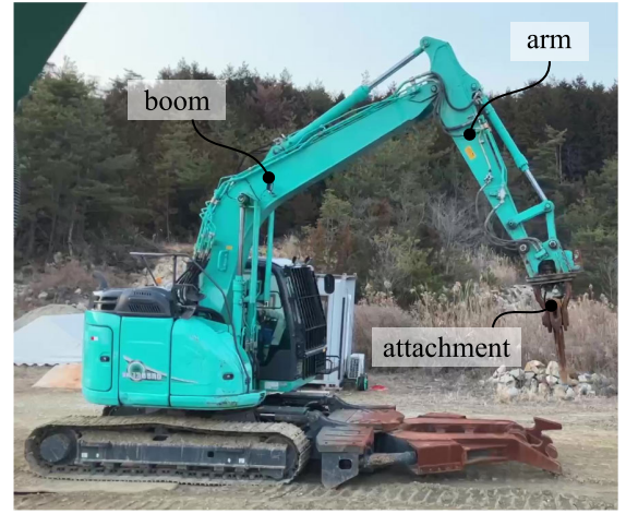
Fig. 12. Kobelco 13-ton class excavator with a shear attachment.
