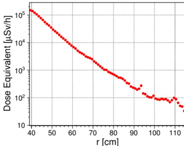
**Borated concrete with 75 cm thickness** reduces rate of dose equivalent (averaged over 1 m in z-direction) to **30  $\mu\text{Sv/h}$**  after 5000 hours of source operation and 1 hour cooling
