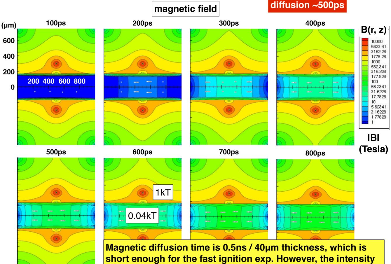
of magnetic field inside cone is reduced by the eddy current.
