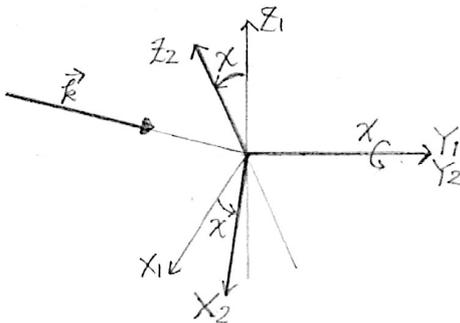
$$[x_3, y_3, z_3] = [x_0, y_0, z_0] \hat{R}, \quad \begin{bmatrix} x_0 \\ y_0 \\ z_0 \end{bmatrix} = \hat{R} \begin{bmatrix} x_3 \\ y_3 \\ z_3 \end{bmatrix}$$
